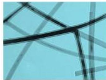
Atomic layer deposition on nanowires, forming a conformal layer of oxide down to 3 nm.
