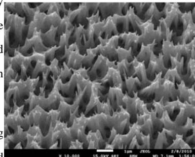
In dye-sensitized solar cells, ZnO functions as a scaffold for light harvesting dyes and as a medium for electron transport. The dyes absorb sunlight and then donate electrons to the ZnO nanowires. As electrons accumulate in the nanowires they diffuse out to the anode. Although ZnO nanowires have excellent electron transport properties, they have lower surface areas than ZnO nanoparticles. On the other hand, ZnO nanoparticles are relatively poor electron transporters.
