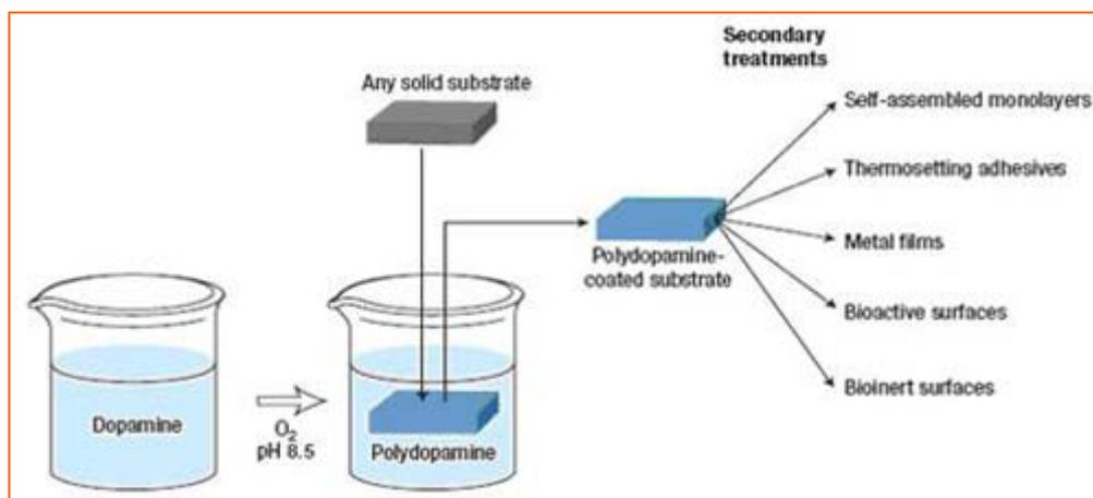
Schematic diagram of the construction of multi-layered films by using polydopamine coating as the interlayer (Picture/WANG Jinqing et al.)
