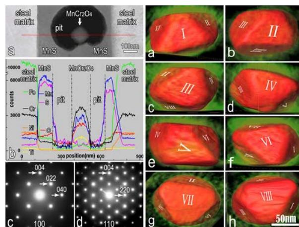
Identification of the spinel MnCr<sub>2</sub>O<sub>4</sub> nano-octahedron around which MnS dissolution occurs in the presence of salt water. (Image by SYNL )
